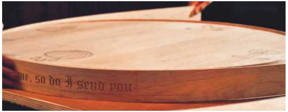
▲ Pic.15 The engraved oak lath being secured in place
